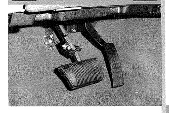
of our Jeep Liberty to mount the remote vacuum pump. Once the pump is securely mounted, the Unified Tow Brake's vacuum lines are spliced into the vacuum lines on the Liberty. While it is true the system does not cut into the towed vehicle's brake lines, it is necessary to splice into the towed vehicle's vacuum system in order for the Unified Tow Brake to work.
