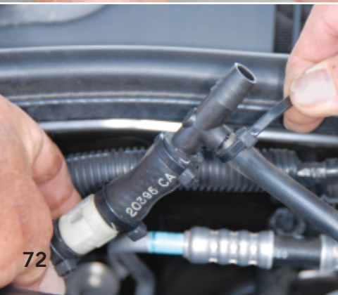
A T-fitting is spliced into the brake system's vacuum line in back of the check valve, allowing the UTB vacuum pump to actuate the dinghy's power-brake system.
