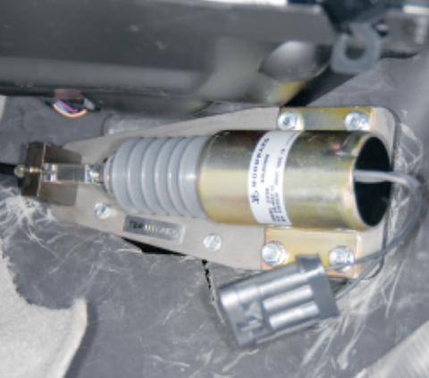
The solenoid that pulls the cable used to depress the dinghy's brake pedal is mounted under the dash on the passenger's side.
