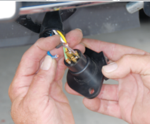
The system's charge and control wires are connected to the six-pin receptacle on the dinghy vehicle that was originally installed when it was wired for towing.
