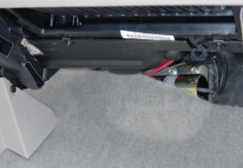
With solenoid and wiring complete, the dinghy's stock carpeting is replaced and secured, virtually hiding this portion of the system.
