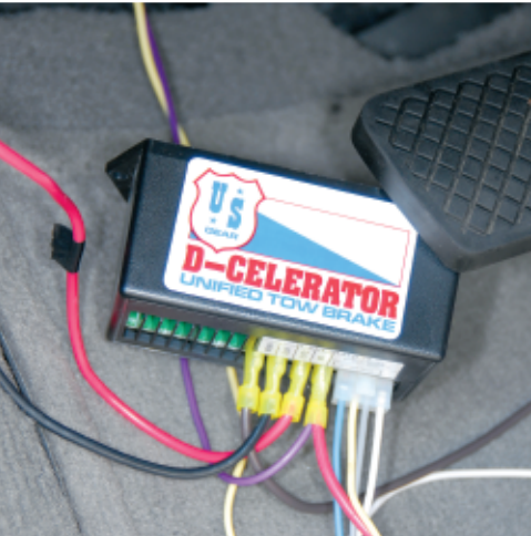
The D-Celerator Unified Tow Brake power module is mounted under the dinghy's dash. All wires will be neatly tied up and away from possible foot snags.
